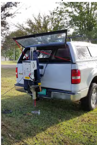
Figure 31: Propelled Energy Generator used as an Active Source.
